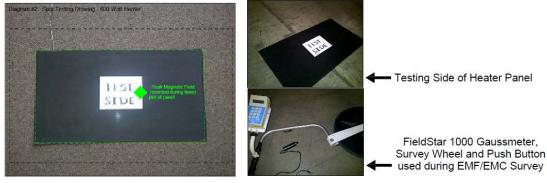
As shown by Diagram #1, the magnetic field recorded atop the sauna heater (with the electrical source placed on the floor) was 0.0 mG with the heater OFF, between 0.12 mG to 0.20 mG in the exact center of the panel after turning the heater ON, between 0.2 mG and 1.5 mG around the center area of the panel after 3 minutes of duration, with the peak magnetic flux density level recorded from the panel at 1.96 mG. The table below summarizes the ramp-up AC ELF EMF magnetic field test:
