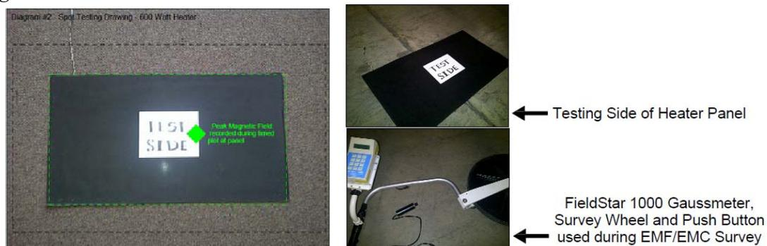
As shown by Diagram #1, the magnetic field recorded atop the sauna heater (with the electrical source placed on the floor) was 0.0 mG with the heater OFF, between 0.12 mG to 0.20 mG in the exact center of the panel after turning the heater ON, between 0.2 mG and 1.5 mG around the center area of the panel after 3 minutes of duration, with the peak magnetic flux density level recorded from the panel at 1.96 mG. The table below summarizes the ramp-up AC ELF EMF magnetic field test:
